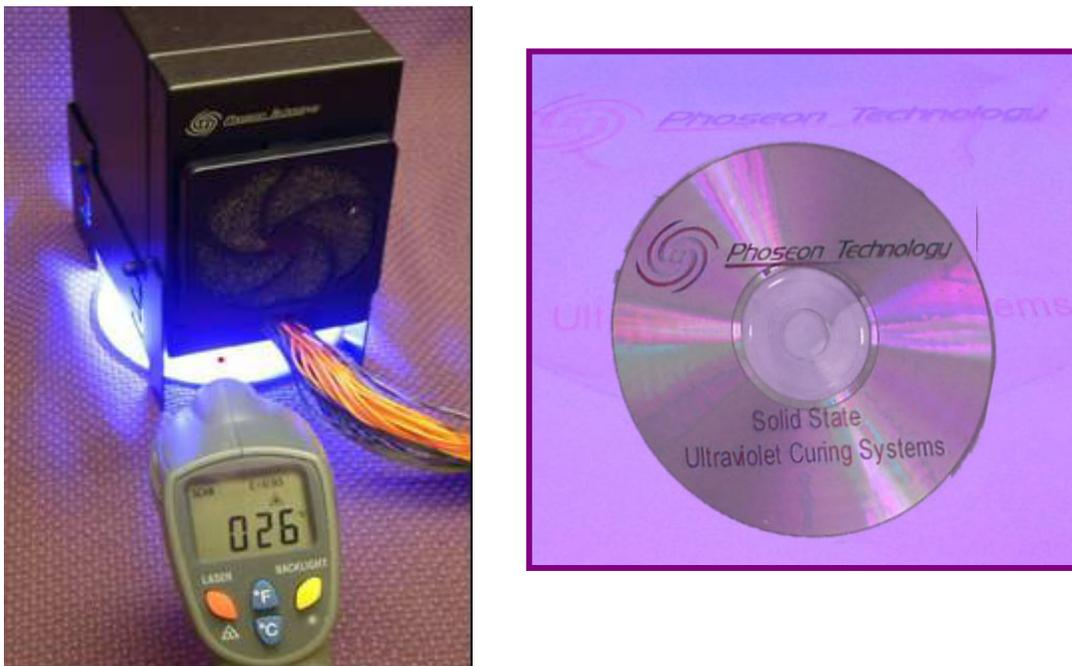
**Figure 9.** Heat sensitive media are an ideal fit with SSD devices, which only heat the media slightly above ambient temperatures during the cure cycle.
