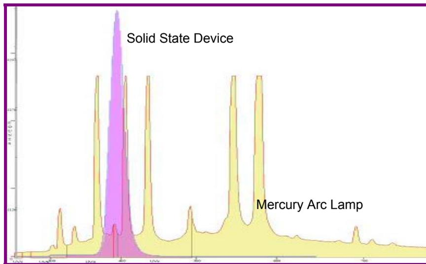
**Figure 6.** Spectral output of a medium-pressure mercury arc lamp and SSD, showing the SSD to be both more intense and have a more narrow band of emission.
