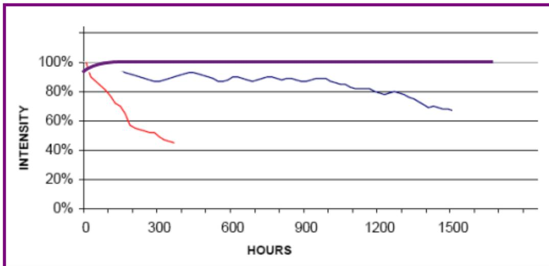
**Figure 4.** Lifetime data for two commercially available arc lamps and SSD Light Source. While no appreciable degradation was observed during this test, > 10,000 hrs is estimated for the SSD.
