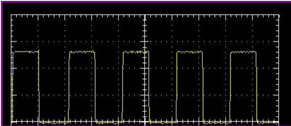
**Figure 8.** SSD sources can provide instantaneous pulses with <1 msec rise times, allowing variable intensities, on/off control, and programmable cure recipes in addition to traditional continuous cures.
