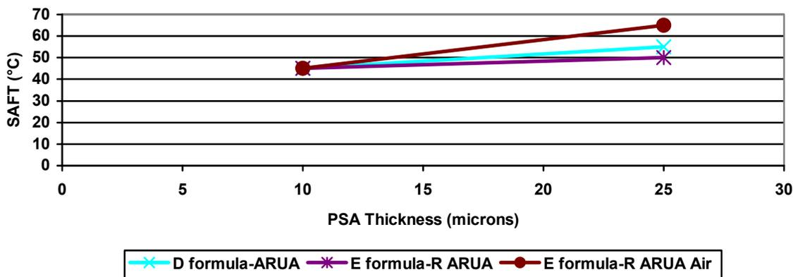
It does appear that as you increase the adhesive thickness, the SAFT will also increase. It is very minimal in these results, which could be an indication of the age of the samples that were tested. It might also be an indication of the adhesive thickness. Since better SAFT has been reported at greater adhesive thicknesses (around 2.0 mil) with similar formulations then maybe a huge improvement is seen between 1.0 and 2.0 mils of adhesive thickness.
