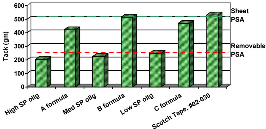
As you can see in [Figure 2](#), the addition of a urethane acrylate oligomer improves the tack over the neat tackifying oligomer. The tacks of the “B” and “C” formulated PSAs are similar to the tack of the Scotch Tape that was tested.
