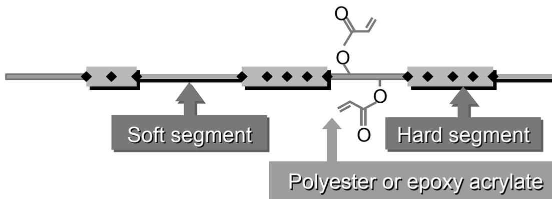
**Fig. 1:** Building blocks of UV-curing polyurethane dispersions
