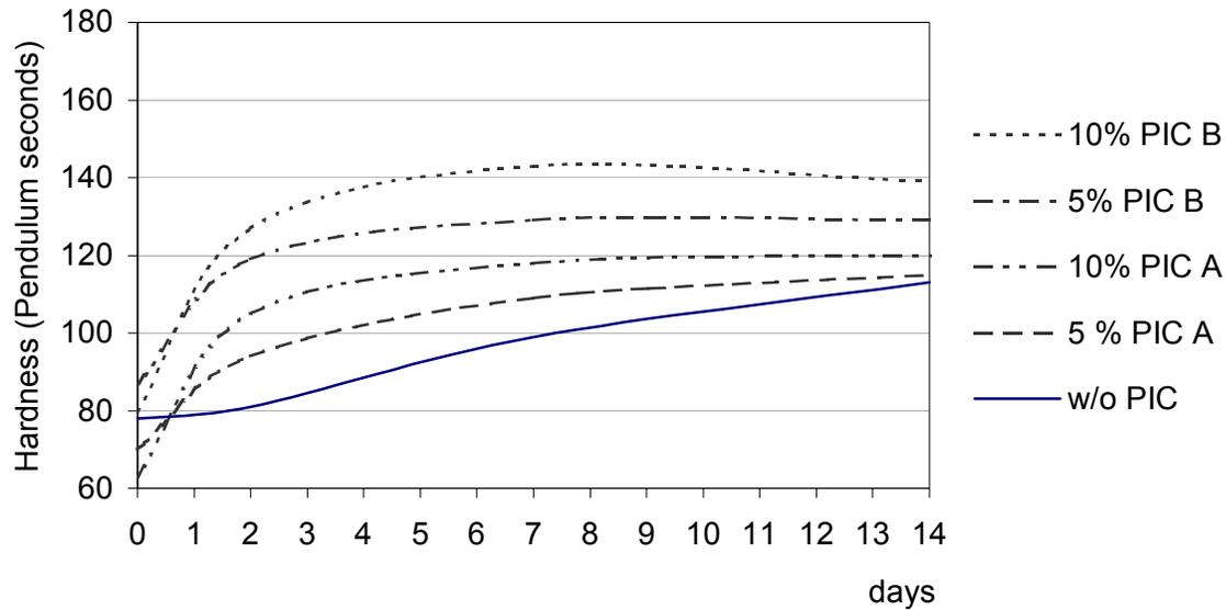
**Fig. IV:** Hardness development of dual cure waterborne UV pigmented coatings
