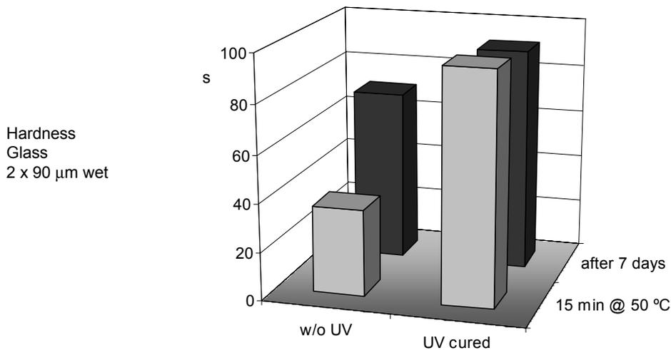
**Fig. II:** Chemical resistance and hardness of PU dispersion-based, white pigmented coating with and without UV-curing.
