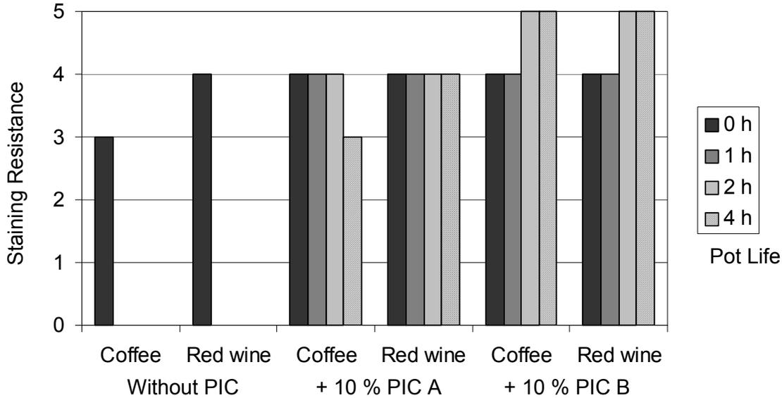
**Fig. III:** Staining resistance of dual cure waterborne UV pigmented coatings DIN 68861 1b, 5 = pass, 0 = fail
