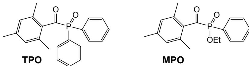
The introduction of bisacylphosphine oxide (BAPO) photoinitiators in the late 1990s' has opened the door for sun light curing and further improved photospeed. Two commercially available products are shown below.<sup>2</sup>
